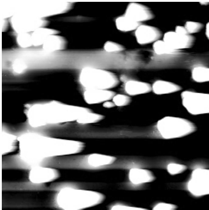
FIGURE 3 Scanning probe micrograph ( 10\ \mu\text{m} \times 10\ \mu\text{m} ) of 1% w/v aqueous gelatin solution with 0.1 M NaCl taken at 25^\circ\text{C} in the tapping mode in presence of 33.3% v/v ethanol. The picture shows gelatin aggregates giving rise to larger clusters of typical size 1000 nm. Tiny particles not clearly seen in the background are single molecules of typical size 30 \pm 5 nm.
